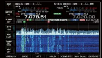
Spectrum scope with waterfall (wide screen setting)
